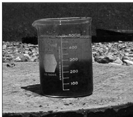
Solids going into the Geotube® container is about 9,000 mg/l.
