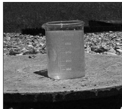
Resulting filtrate weeping out of the Geotube® container at about 8 mg/l permitted the filtrate to discharge directly to the river.
