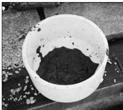
Sludge from inside the Geotube® immediately begins to dewater.
