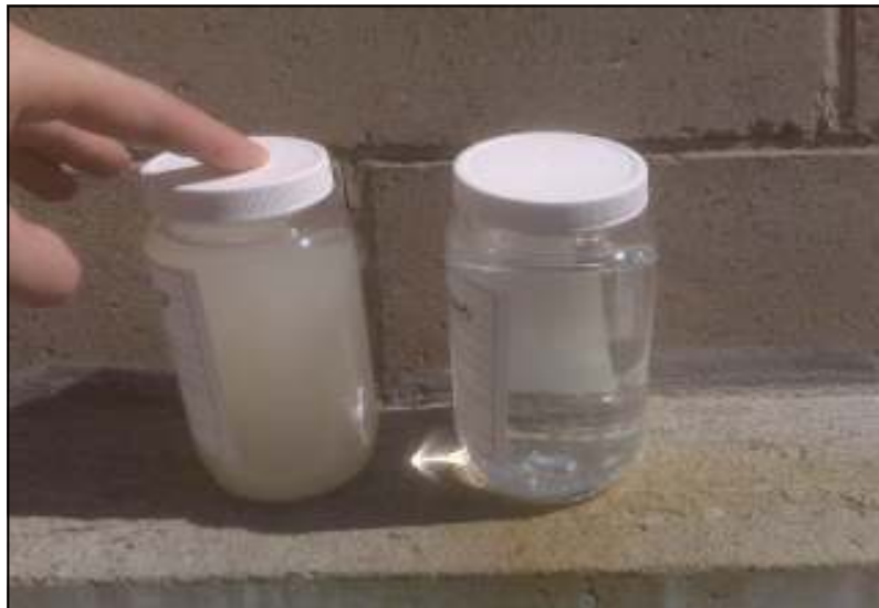
On the left is wash water from an Ontario cheese factory prior to being dewatered by the Geotube ® technology. On the right is wash water after having been dewatered by the Geotube ® technology.
