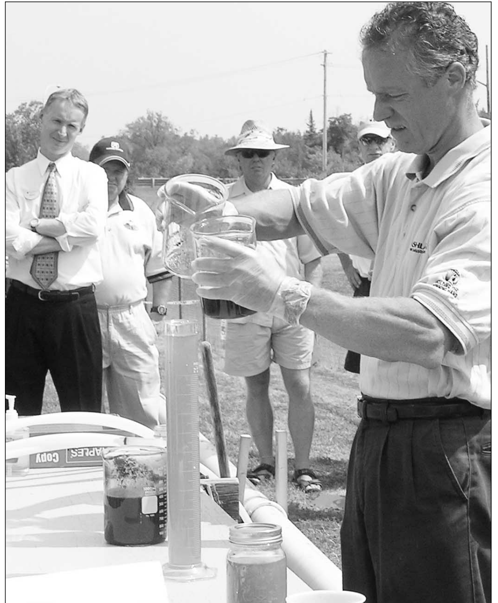
Paul Lefevbre, district manager of Ashland, Drew Industrial gives a demonstration on how adding polymer to the sludge speeds up the separation process.
